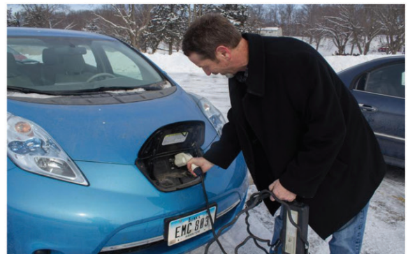
Nissan Leaf owner Rand Faaborg demonstrates how he attaches the electric cord to his car. The other end can be plugged into any standard 110-volt outlet. AMY MAYER / HARVEST PUBLIC MEDIA
